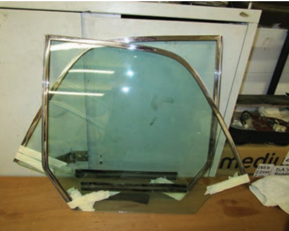
The side windows re-fitted in their frames and ready to go back in the car.
