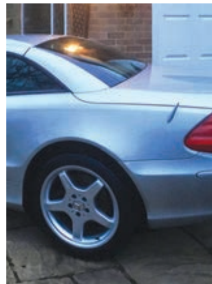
The repaired wheel arches on the SL500 remain perfect after five years. Inner box sections and the rear valance were removed to facilitate the work at £300 per side.
