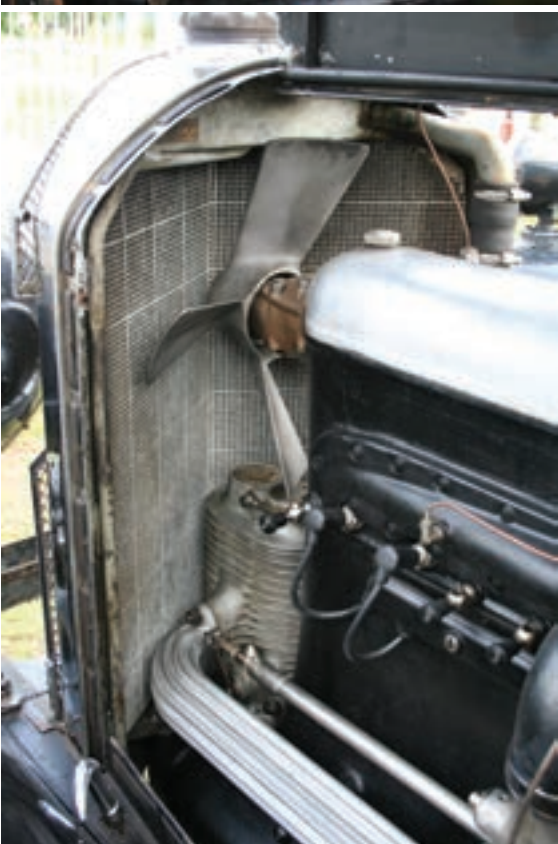
The 1928 630 of Antonio Turroba from Spain. Note the V-shaped radiator and cooling fan.
