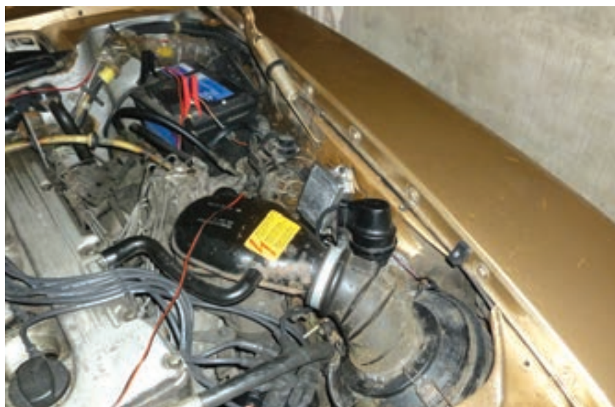
The ignition control unit (a silver coloured box) is located at the top of the nearside inner wing just ahead of the battery.
