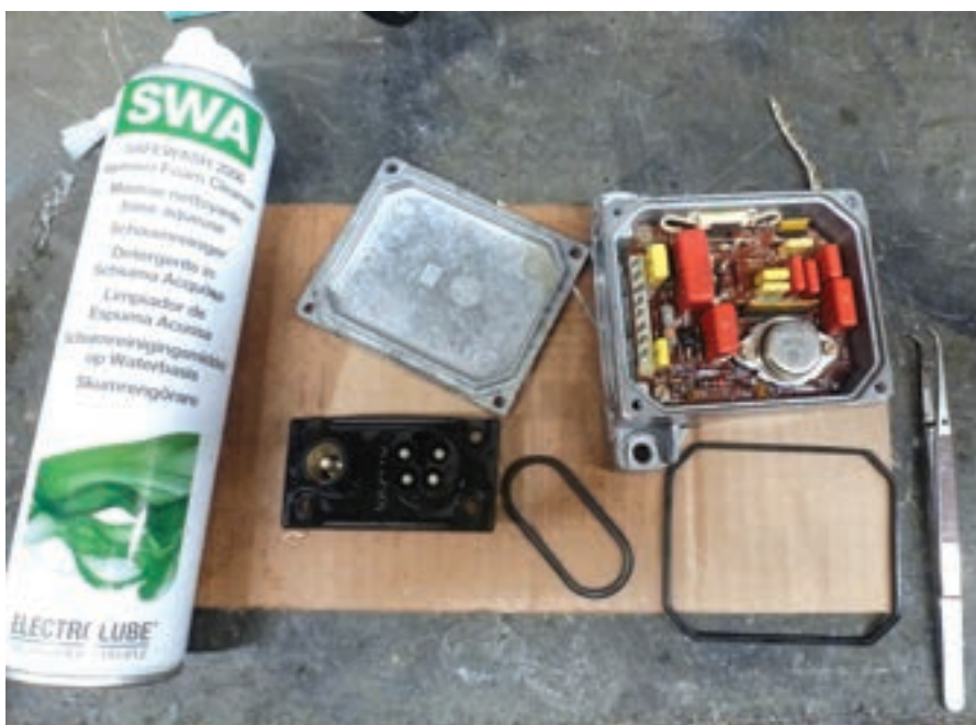
Safewash was used to clean the PCB after soldering. The re-assembled control unit is on the right and its connector block in the centre.
