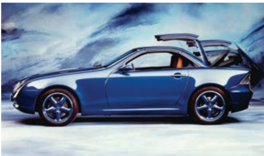
A graphic showing the operation of the Vario roof.
