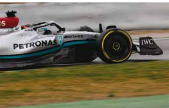
One of the most noticeable changes are the bigger wheels. This is George Russell's car in Barcelona.
