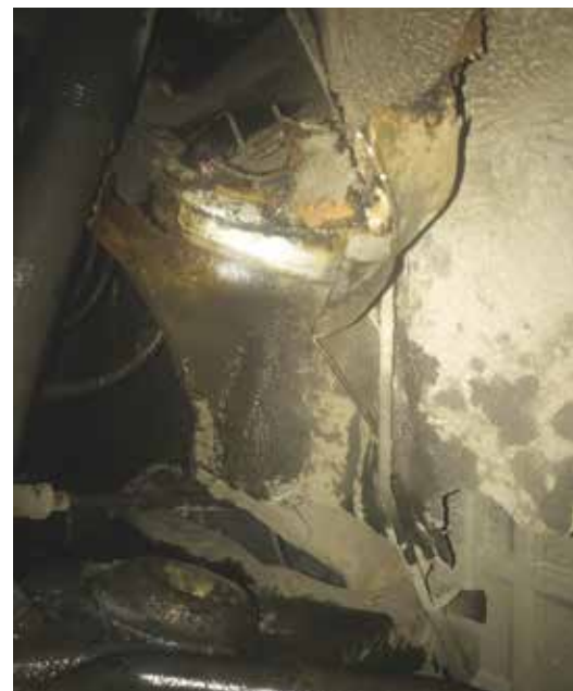
Spring perch split, a weak point on many DaimlerChrysler cars.
